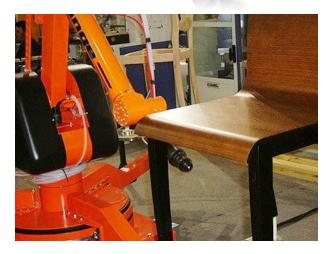
The AL4 automatic electrostatic system enables to paint particular metal, wood, structures and more with considerable savings of paint consumption and increased production speed. Suitable for carpentry in general or wood production, It can also spray high viscosity or abrasive paints materials with exceptional finish results.
